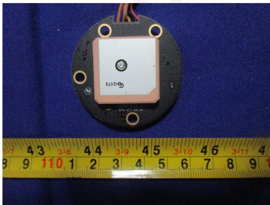
EUT –GPS Bottom & Antenna View
