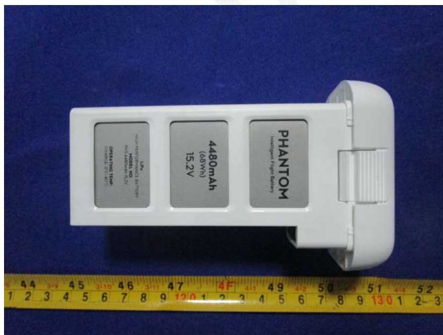
EUT – Battery Top View
