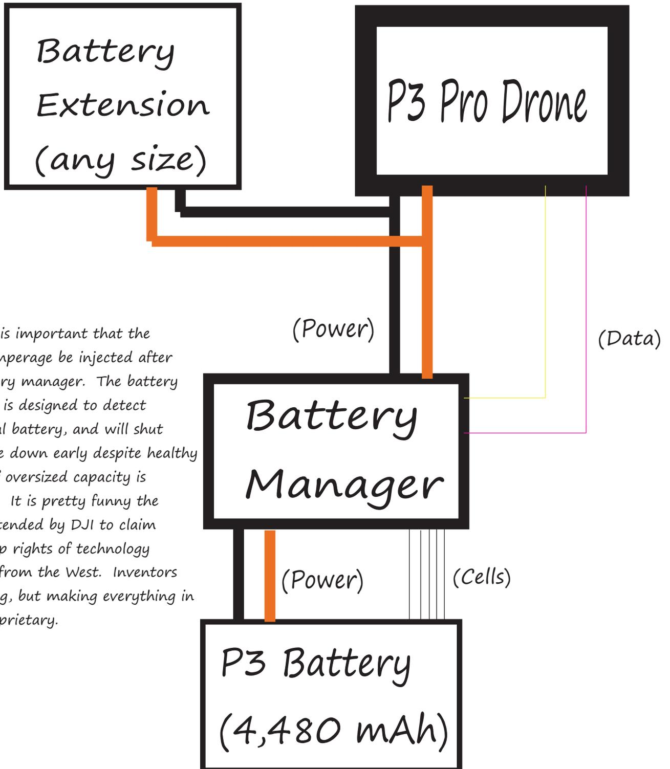
*Note: It is important that the added amperage be injected after the battery manager. The battery manager is designed to detect additional battery, and will shut the drone down early despite healthy voltage if oversized capacity is detected. It is pretty funny the effort extended by DJI to claim ownership rights of technology hijacked from the West. Inventors of nothing, but making everything in sight proprietary.*
